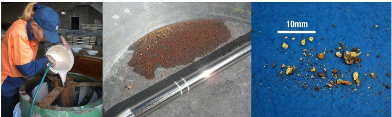
Figure 1a: Processing aircore samples with Knelson Concentrator.
