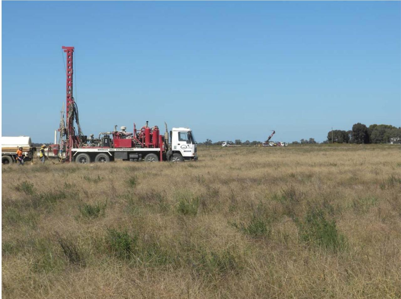
**Figure 3 – Aircore Drill Rig (foreground) and Diamond Drill Rig (rear right) in operation at Four Eagles Gold Project (March 2011)**
